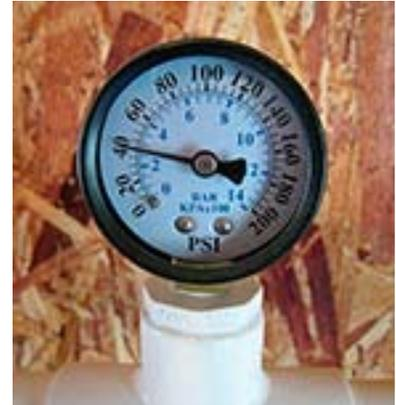
**Water pressure at the control room needs to be about 40 psi under maximum demand flow. If the water system cannot maintain good pressure under maximum demand, there is a problem to be found and fixed.**
